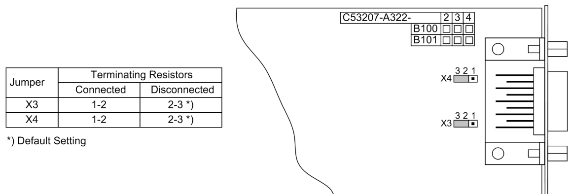
Figure 3-8 Position of the jumpers for configuration of termination resistors of the PROFIBUS FMS and PROFIBUS DP interface
