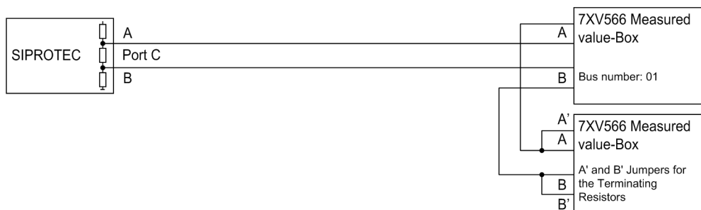
Figure A-20 Electrical connection (RS485) of two measurement boxes
